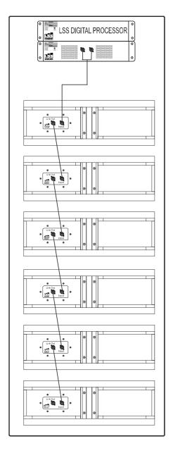
HDA24 system operating mode is only Bi-Amp (LF 1- 1+; HF 2- 2+) and needs an external digital processor with custom setup provided by LSS. If your amplifier can manage a 2 Ohms Load and has sufficient power, it is possible to connect a maximum of 6 speaker in parallel (total impedance will be 2 Ohms).
