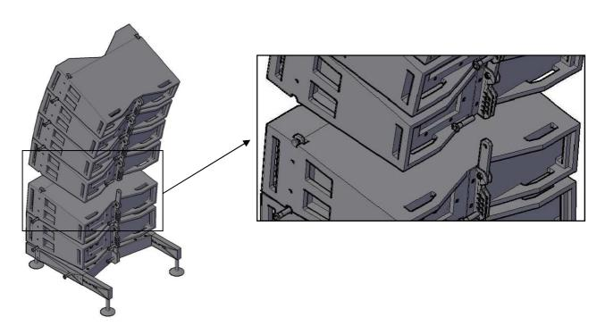
The regulation holes of the bracket allow to choose the desired inclination of the top speaker than the bottom speaker.
