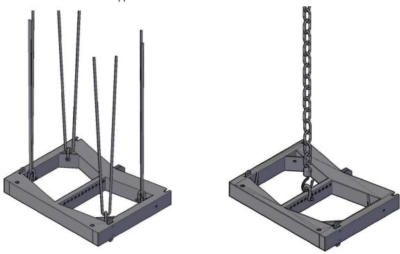
Suspending the bumper from holes for suspension and regulation of inclination, it is possible to determine the inclination of the entire system. Inclination value depends from hole and speakers used because of varying the number of speakers, change the center of gravity, so for an exact operation use an inclinometer.
