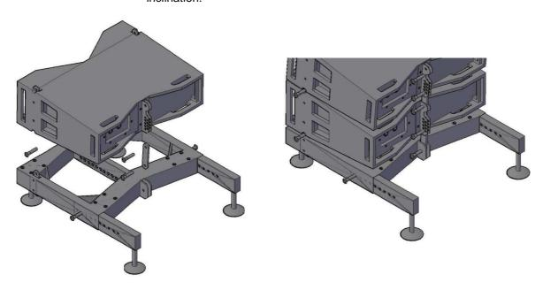
In case of installation in Flying mode, use the bumper without extensible bars and feet, attach the speaker to the sides via connecting bracket, then connect the rear bracket adjusting the inclination.
